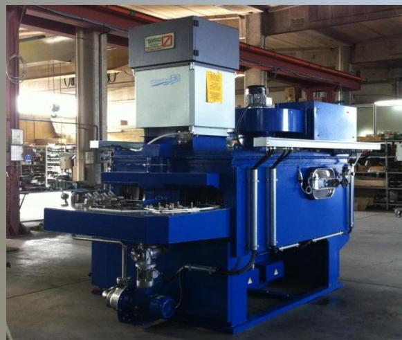
Tunnel with **CIRCULAR CONVEYOR** are particularly recommended for spray treatments of mechanical pieces of small and averages dimensions. The system of transport is composed by a rotating table that, moving around a central pivot, transports pieces holder satellites in the different stage of the treatment.
